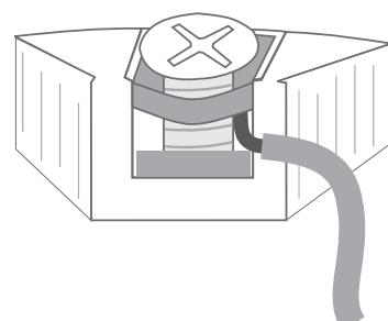
Wires must be mounted between the metal plates.
